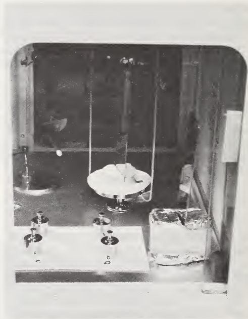
Figure 2: View of weighing chamber with a parallelepiped weight on balance pan.
